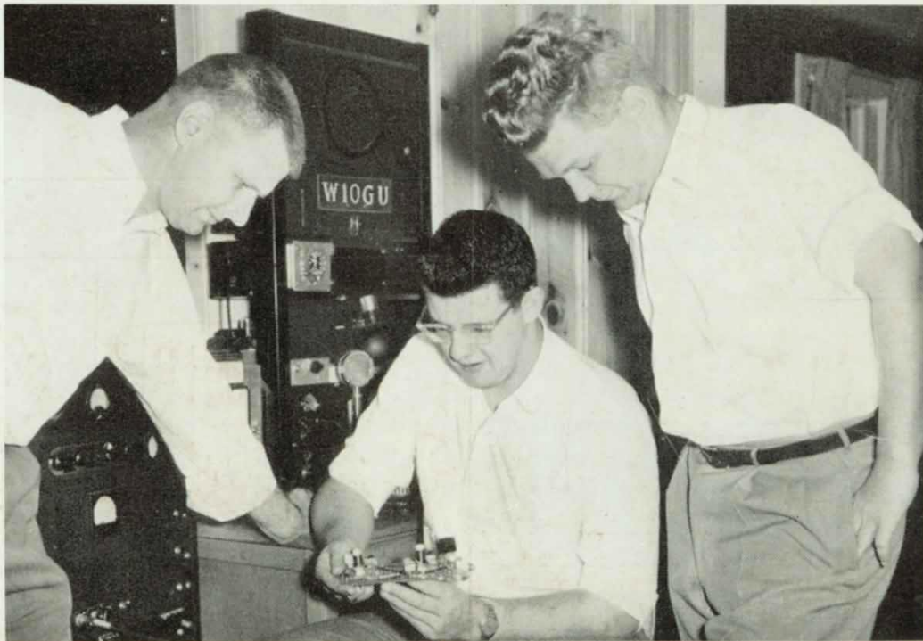
Al Hankinson, Dick Wright and Gus Fallgren compare their mite-sized transmitter with standard transmitter in background. Drastic reduction in size was achieved by using two Raytheon transistors.
